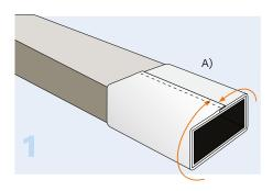
Perimeter wrapping of Tekno- Fire section **A)** on channel. The joint overlap Is longitudinal.
