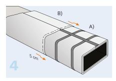
Tekno-Fire section **B)** cut to measurement and arranged in sequence, as indicated inpoint 1), with the perimeter joint overlap (5 cm) between the two consecutive sections.
