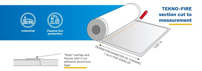
The process begins with a TEKNO-FIRE section cut to measurement and wrapped around the perimeter of the system.
