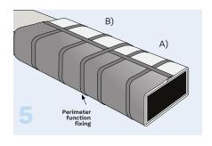
Fixture with aluminium adhesive tape of section **B**), according to points 2-3). Complete fixture with the same tape on the overlap of the perimeter joint between the two sections **A-B**).
